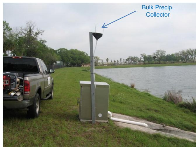
Figure 2-4. Inflow Monitoring Equipment at Site 3.
