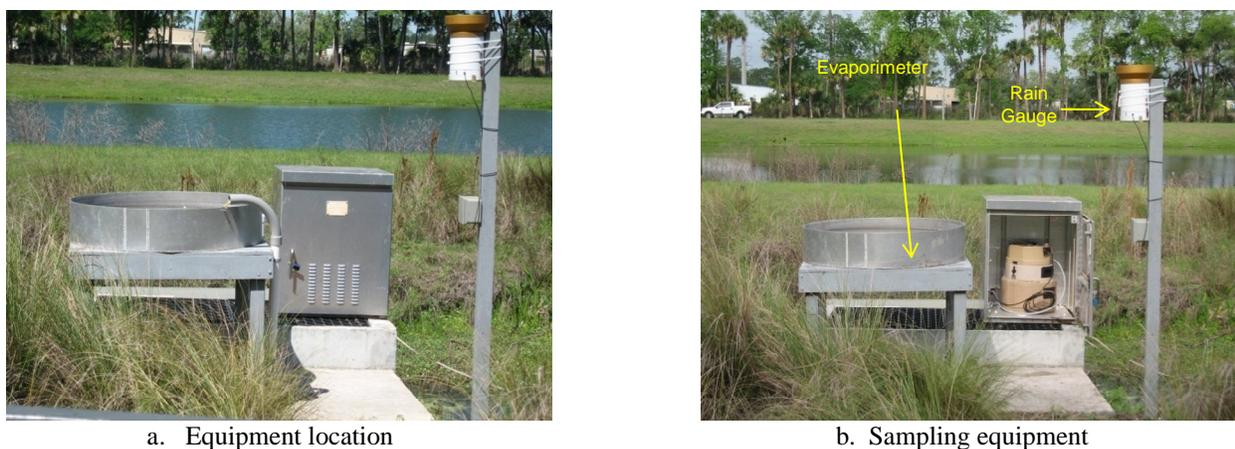
Figure 2-5. Inflow Monitoring Equipment at Site 4.
