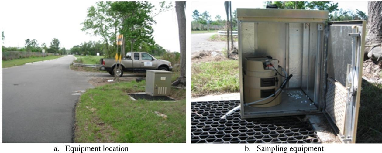
Figure 2-3. Inflow Monitoring Equipment at Site 2.
