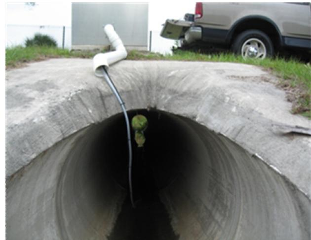
d. Sample Intake and Flow Probe Extended into Pipe
