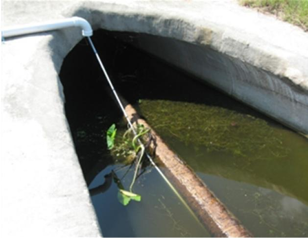
a. Floating palm tree relocated sample intake and flow sensor
